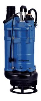
Solidpump TBD agitator series are cast iron heavy-duty slurry / sand pumps using TBZ pumps as a base. TBDE pumps are equipped with agitators that assist smooth suction of the pumped media.
